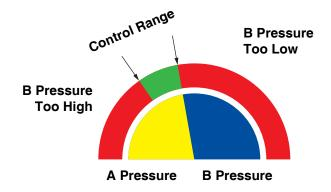
Fig. 57. A/B Control Range with Properly Sized Restrictor
